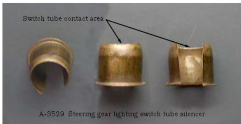
Three views showing the shape of the "silencer".
