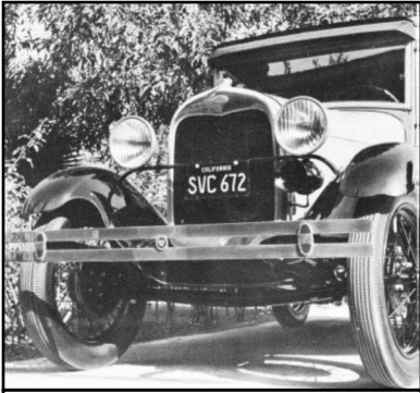
Bumper with flat rounded, open end, without the usual bolt, is one of the more obvious features of a true "early bird." Also notice round center bumper clamp with Ford script and "made in USA" - same as Model T.
