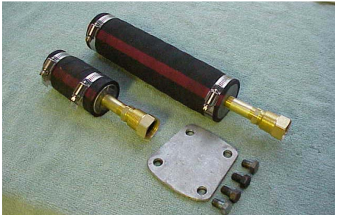
Shown above are the two adapters and the water pump blanking plate. The long hose is the upper (larger diameter) hose. The short hose is the lower (smaller diameter) hose.
