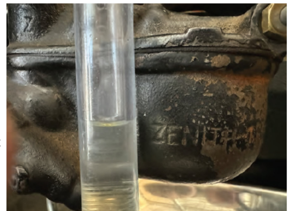
(Below) The fuel level was 1 inch below the casting top!
