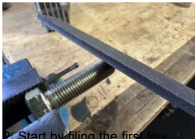
2. Start by filing the first few threads to create a starter thread or pilot depending on what you need
