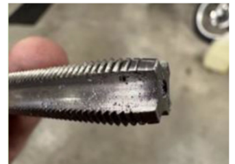
Notice the lack of a pilot to help center the cutting tap, and also the cutting edges to remove material
