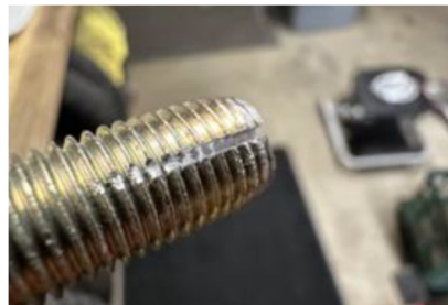
3. Using a hacksaw to slice a relief for chips or other debris can make the job easier
