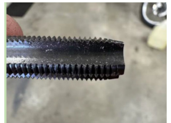
A cutting tap has a shape meant to form new threads
