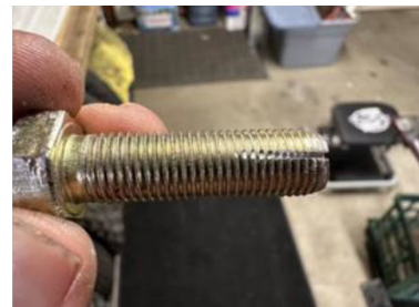
4. A thread chaser, made at home in 10 minutes
