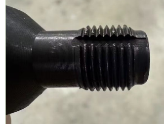
Thread chaser. Notice the distinct shape that is much less aggressive than a tap.
